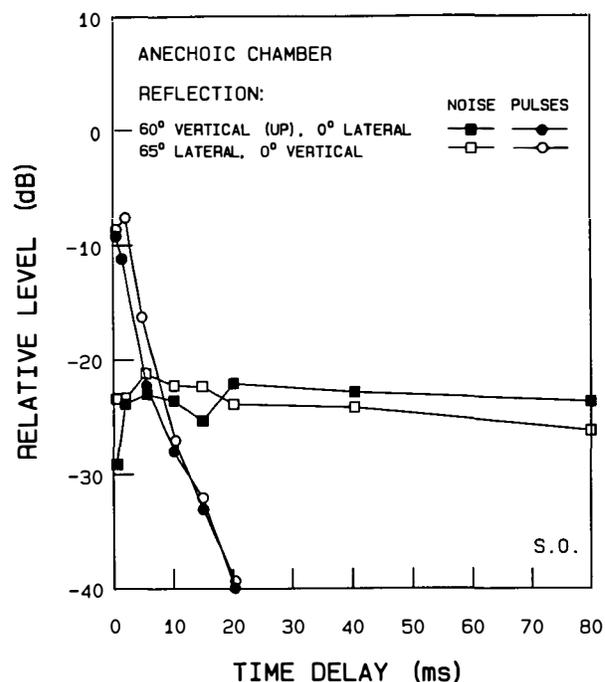
Fig. 2. Absolute thresholds for single vertical reflection (solid symbols) and single lateral reflection (open symbols) using two different types of signals: pink noise (squares) and pulses at 2/s (circles). Anechoic listening.
