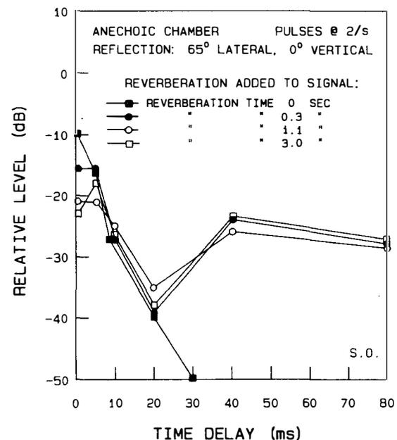
Fig. 7. Absolute threshold for lateral reflection, using pulses at 2/s that are processed with increasing amounts of reverberation using a Yamaha DSP-1. Program—chamber; initial time gap—5 ms,  $R_{160} = 0-3.0$  s. Anechoic listening.
