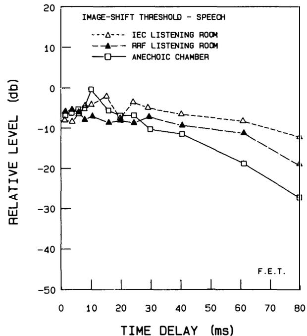
Fig. 12. Using the exact experimental conditions as in Fig. 11, here image-shift threshold is shown, indicating the minimum level at which the lateral reflection is perceived to cause a spreading or shift in localization of the auditory event associated with direct sound.
