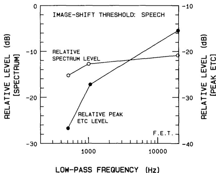
Fig. 17. Image-shift thresholds for 65° lateral reflection that has been low-pass filtered at 20 kHz, 1 kHz, and 500 Hz, all delayed by 30 ms. Measured level of reflection relative to broadband direct sound is shown in two ways. Scale on left shows relative spectrum level of reflected sound at threshold, in the manner used throughout this paper. Scale on right shows corresponding relative levels as indicated by the appropriate peaks in an ETC display. Anechoic listening.
