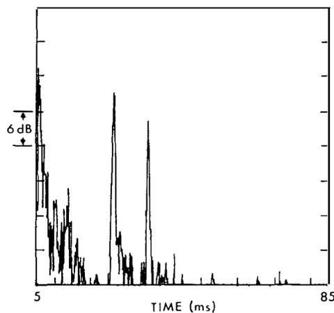
Fig. 14. ETC measured at the listener's head location in anechoic chamber, showing direct sound followed by  $-4$ -dB side-rear reflection at 20 ms and  $-9$ -dB lateral reflection at 30 ms.
