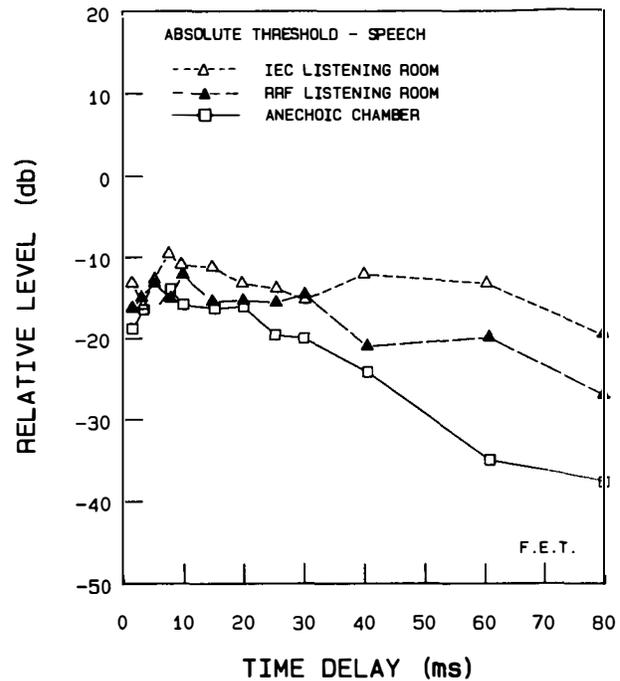
Fig. 11. Absolute thresholds for single lateral reflection ( $65^\circ\text{H}$ ,  $0^\circ\text{V}$ ), using speech, measured in three different rooms that range from total absence of reverberation (anechoic) to room with some reverberation (RRF) and a normal room with relatively strong early reflections and moderate reverberation (IEC).
