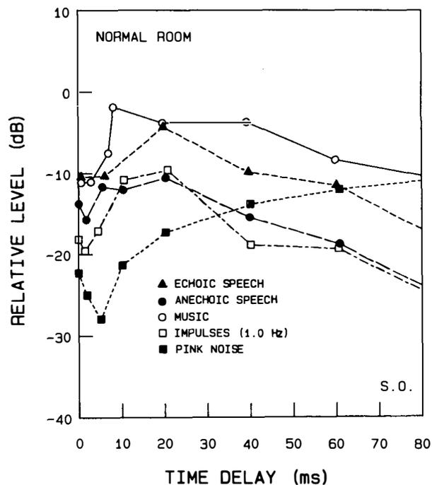
Fig. 13. Results taken from a previous study of detection of resonances [5], showing absolute thresholds for delayed broadband repetition added to signal and reproduced through single loudspeaker in the IEC room, using a variety of different signals.
