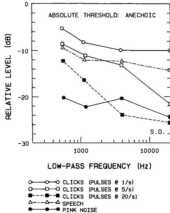
Fig. 16. Absolute thresholds for lateral reflection (50°H, 0°V) that has been low-pass filtered at 20 kHz, 4.4 kHz, 1.2 kHz, and 600 Hz. Reflections were all delayed by 4 ms and signals ranged from discontinuous (pulses at 1/s) to continuous (pink noise).
