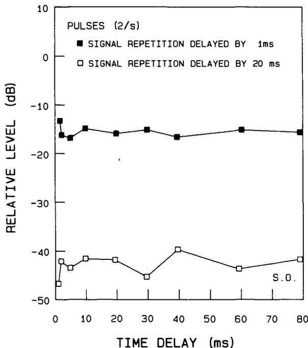
Fig. 9. As Fig. 8, but with simulated wall reflection at  $-3$  dB incident from  $65^\circ H, 0^\circ V$ . The signal was pulses at 2/s.
