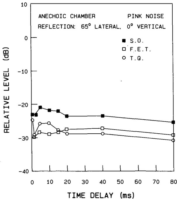
Fig. 3. Absolute thresholds for single lateral reflection shown for three listeners, using pink noise as the signal source. Anechoic listening.
