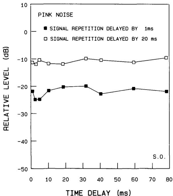
Fig. 8. Thresholds for single repetition in signal path (simulating a reflection in a single channel) in the presence of a vertically incident room reflection ( $45^\circ V, 0^\circ H$ ) at different time delays. The simulated ceiling reflection is at  $-3$  dB relative to the direct sound. Thresholds were determined for two repetition delays, 1 ms (e.g., reflection from a lectern or music stand) and 20 ms (e.g., ceiling or wall reflection). The signal was continuous pink noise.
