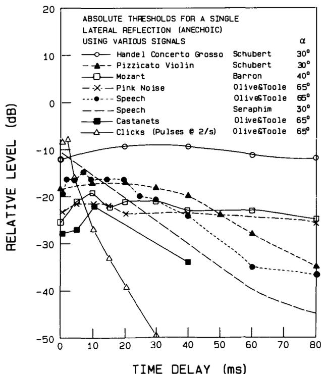
Fig. 6. Comparison of data from this study and from Schubert [8], Barron [10], and Seraphim [6] showing absolute thresholds for single lateral reflection using a variety of natural and artificial signals. All studies used anechoic listening conditions, with slight variations in the horizontal angle of incidence  $\alpha$  selected for lateral test reflection.
